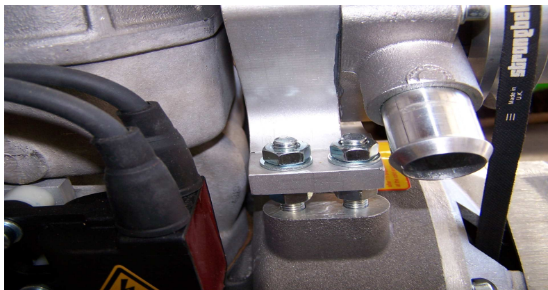
Figure 8.2 Lock nut locations
