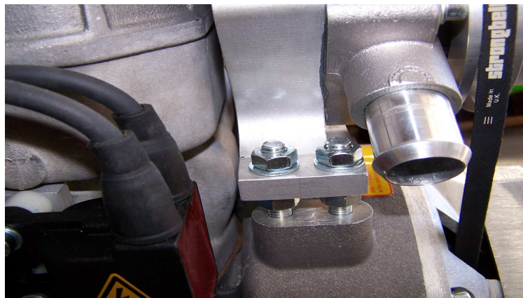
Figure 8.2 Lock nut locations
